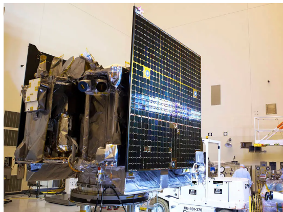
Figure 4.13: Illumination testing for OSIRIS-REx solar arrays ( in [21]) .
