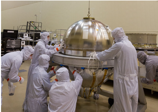
(a) Propellant tank in a rotation fixture to facilitate ground processing ( in [29]).
